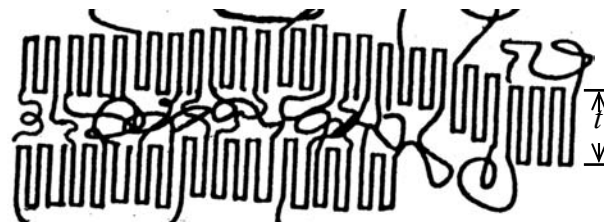
Figure 1. Schematic illustration of the lamellar structure of a semicrystalline homopolymer. Straight lines represent crystal stems, while curving lines represent amorphous sections of polymer chain. Crystal thickness t is typically of order 10 nm.
